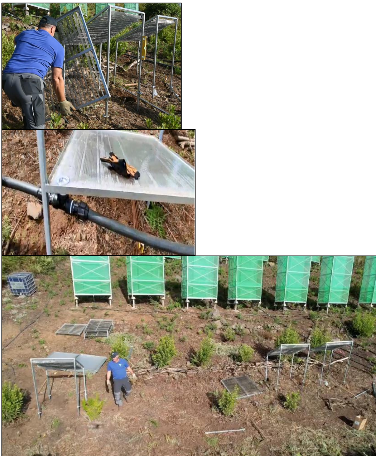
Fig. 53. Field deployment of i-FWC 2.0 units below the t-FWC in El Pinillo (Valleseco, Gran Canaria).
