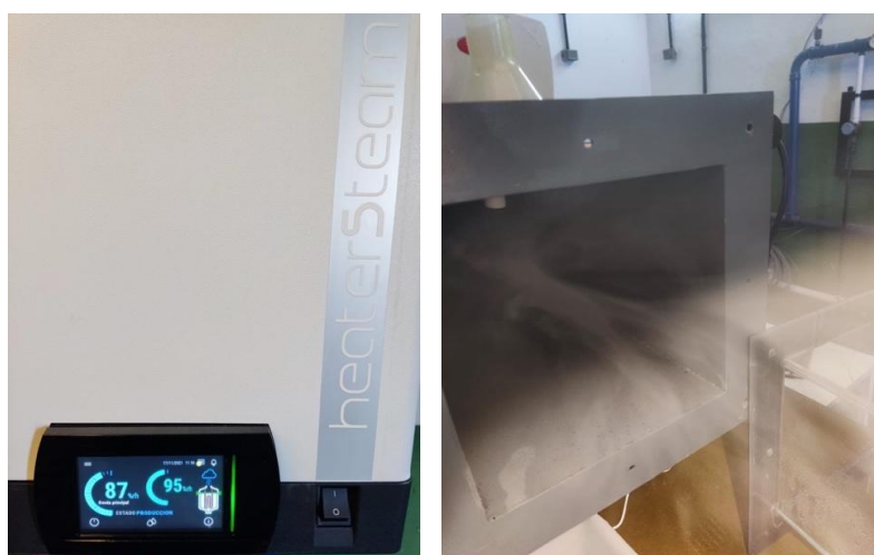
Fig. 20. Steam humidifier acquired to be able to reproduce inside the wind tunnel foggy conditions close to those present in the field. Close-up view of the heaterSteam (left). Water
