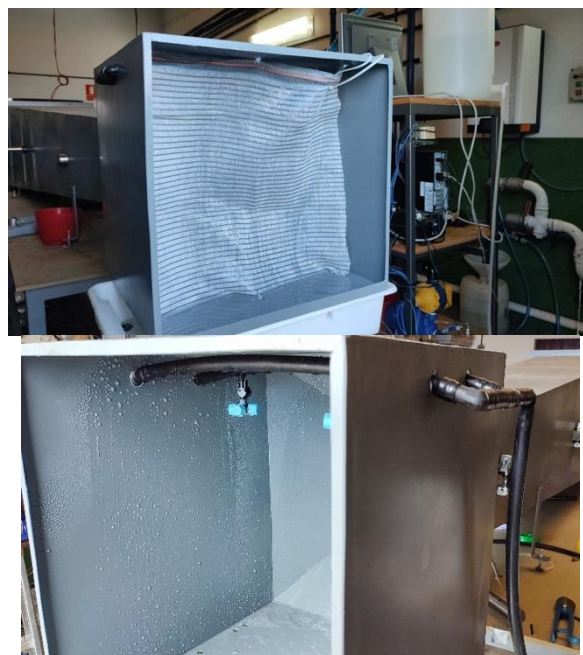
Fig. 19. Adiabatic humidifier constructed at ICIA placed at the entrance of the wind tunnel. In the right hand side photo, the shading screens have been removed to show the sprinkling system used to wet and cool the passing air.
