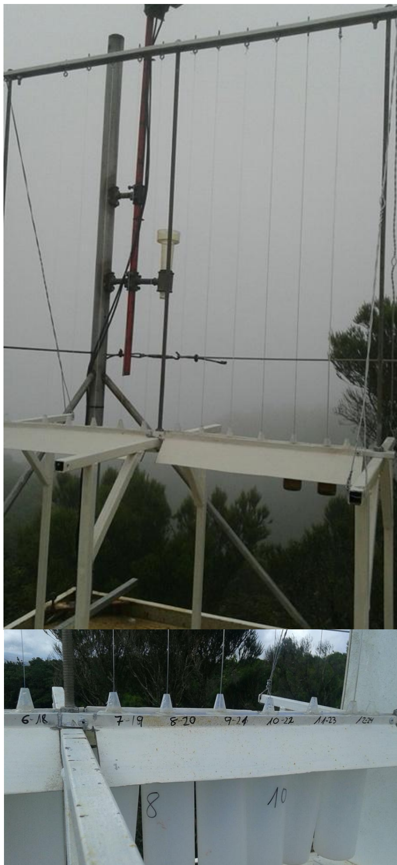
Fig. 2. Set-up of single nylon filaments of varying diameter (top) and detail of collecting bottles (bottom) displayed in the Taborno field site.
