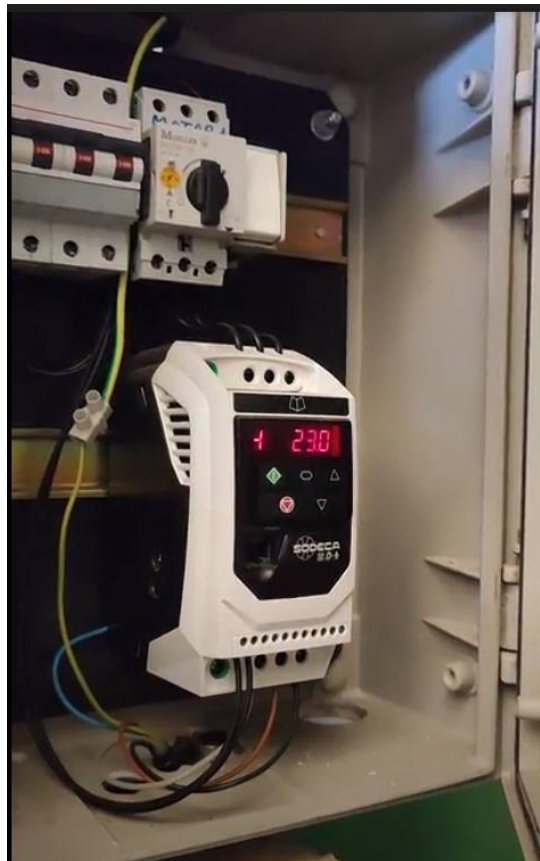
Fig. 11. Fan and variable frequency drive (AFD) for controlling the air velocity inside the wind tunnel.
