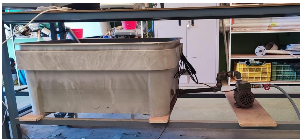
Fig. 17. Recirculation system showing water pump and storage tank.
