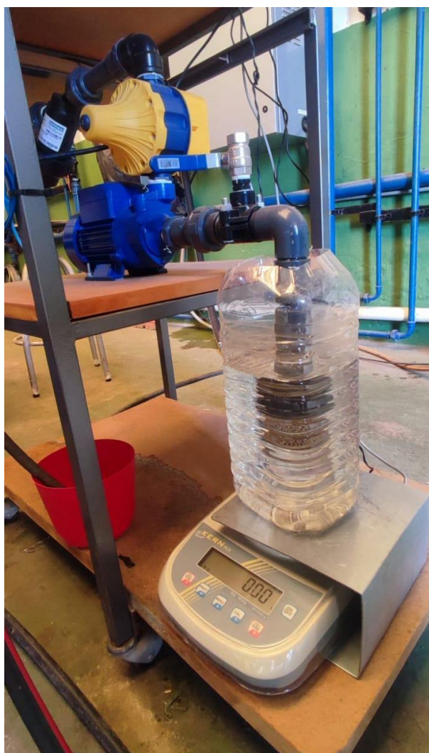
Fig. 16. Water pump system installed at the inlet of the ultrasonic humidifier.
