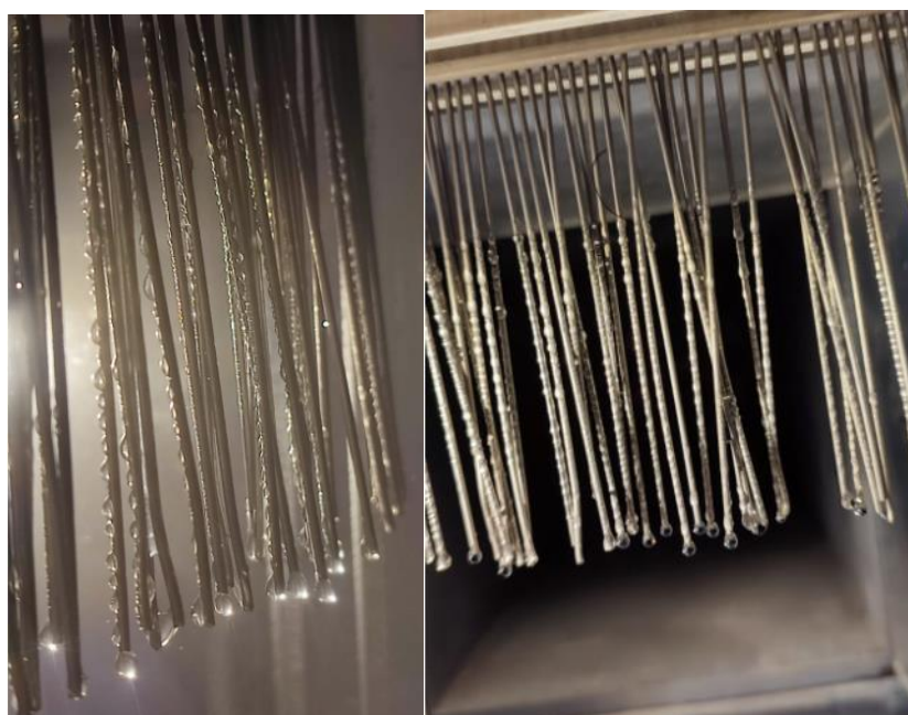
Fig. 49. Wind tunnel experiment with an equivalent arrangement of metallic strings to that of the anti-clogging screen.
