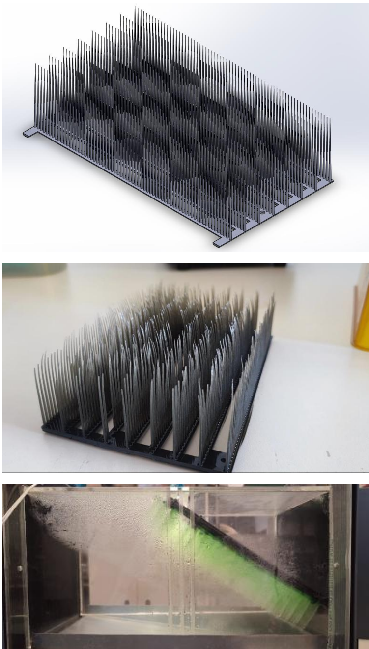
Fig. 46. From top to bottom: final FWC prototype designed, 3D printed and tested in the wind tunnel.
