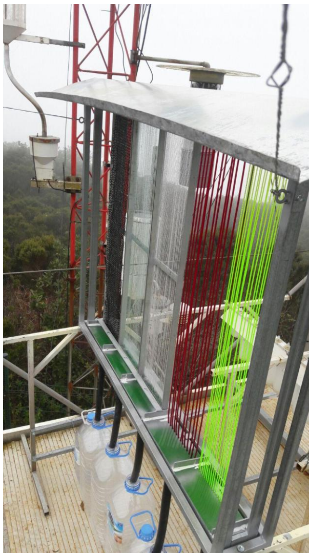
Fig. 4. Experimental set up of harp-like filament arrangements of varying diameter and constant shading coefficient, SC=30% displayed in Taborno experimental site.
