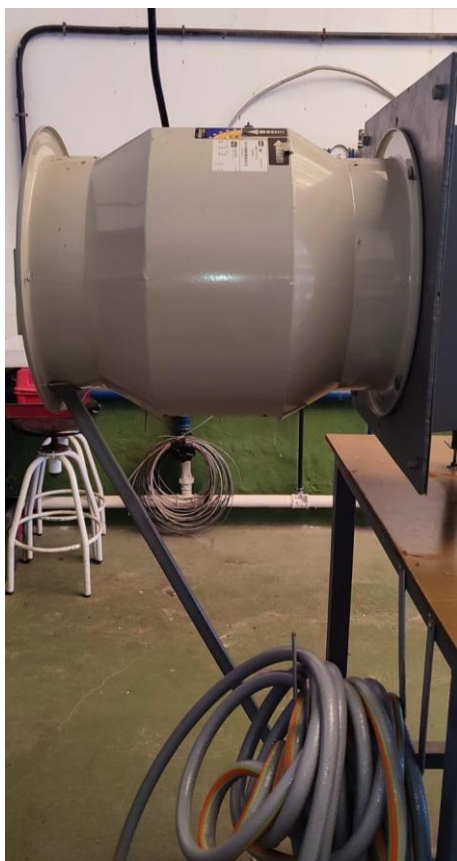
Fig. 11. Fan and variable frequency drive (AFD) for controlling the air velocity inside the wind tunnel.
