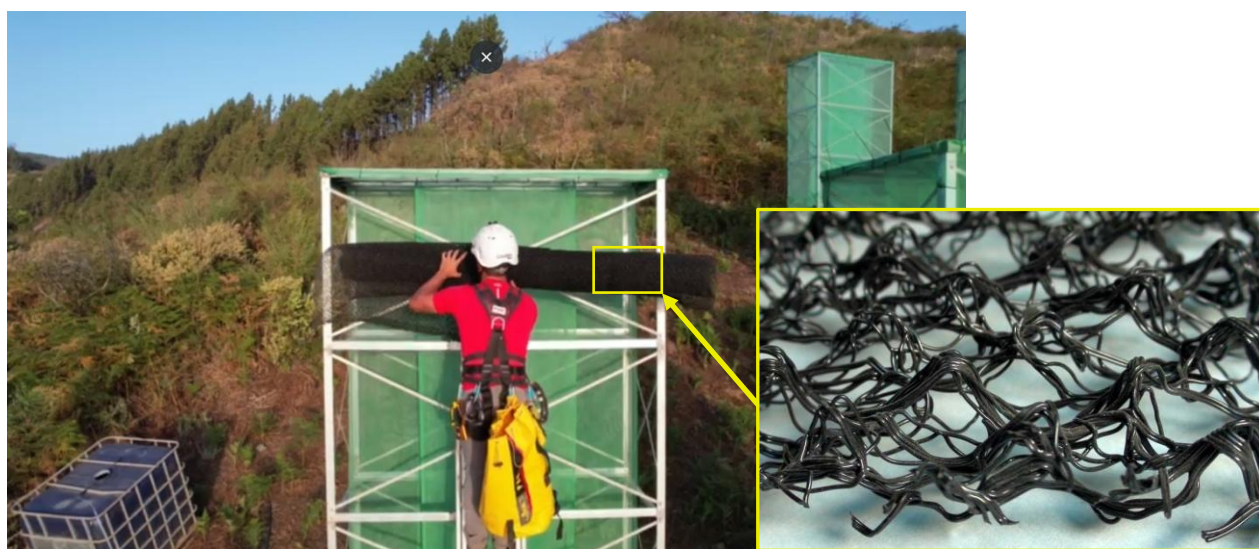
Fig. 57. Traditional fog water collector (t-FWC) where the mosquito screen (green) is being replaced with a volumetric textile (v-FWC).
