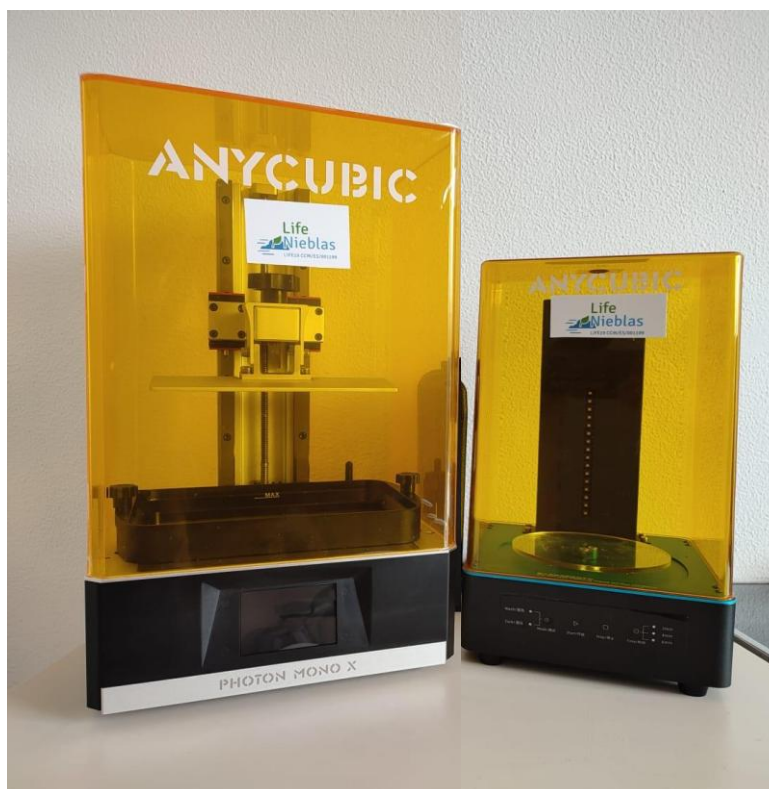
Fig. 22. 3D printer (left) and drying chamber of the resin printed models (right).
