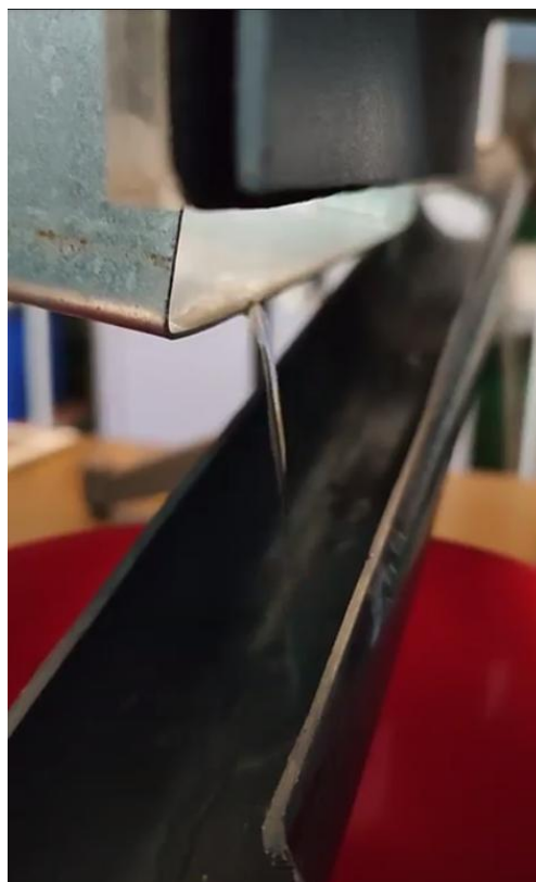
Fig. 44. Detail of collecting ramp, dripping in the gutter below, fabricated to replace the lower side of the test chamber in the wind tunnel.
