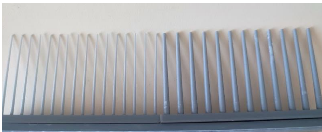
Fig. 28. Some examples of 3D printed screen models manufactured to evaluate the optimum geometrical filament parameters.
