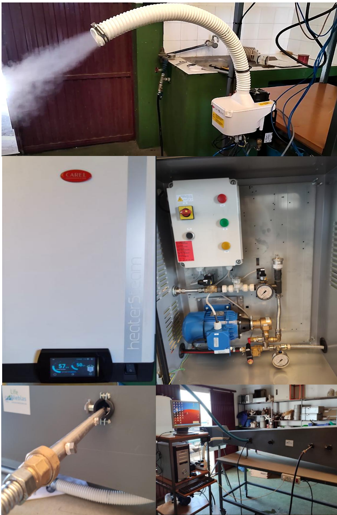
Fig. 15. From top to bottom: Ultrasonic fog generator, steam humidifier, high pressure atomizer, duct distributor with spraying nozzles and overall view of the instrumented humidification cone of the wind tunnel.
