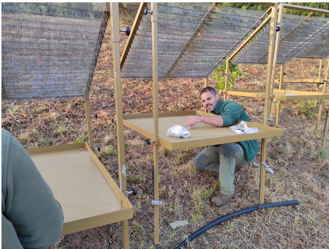
Fig. 55. The upgraded version of the fog water collector (i-FWC 2.1) being installed in the field, showing the improved collecting tray.
